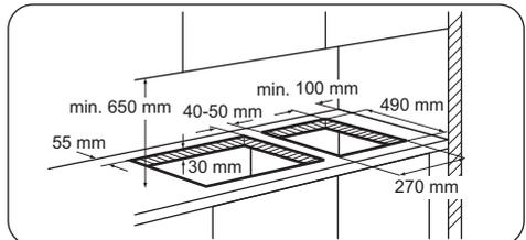
If several 30 cm hobs are to be installed side by side into the same cut out, an assembly kit including a support side bracket and supplementary seals is available at our Authorised Service Centres. The relevant installation instructions are supplied within the kit package.
