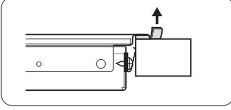
Fit the hob in the cut out and push it down until comes in contact with the kitchen top surface. then remove the excess sealing.
